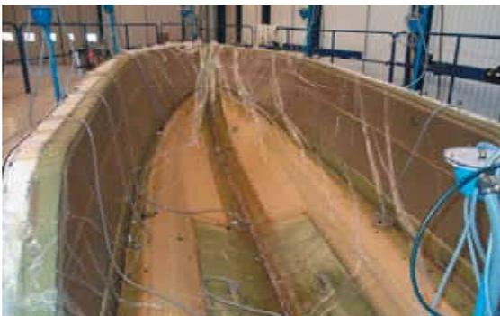
When the reinforcement package is fully impregnated with resin, the resin feed is cut off. Still under vacuum, the laminate is left to cure.
