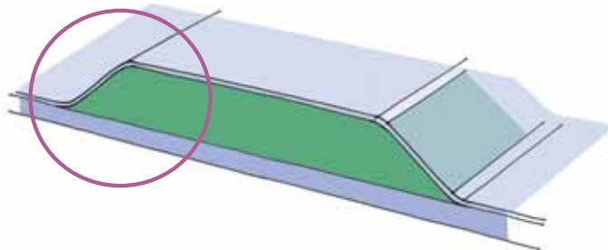
In many cases it will be required to drill/ nail holes in the core, to ensure the resin can flow with the same speed on both sides of the sandwich core.
