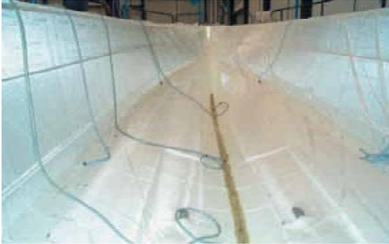
A normal, female Hand lay- or Spray up (HLU/ SU) mould can be easily modified for Vacuum Foil Infusion by extending the flange to enable clamping/ sealing of the foil, and possibly by adding a peripheral gate or channel for the resin feed.
