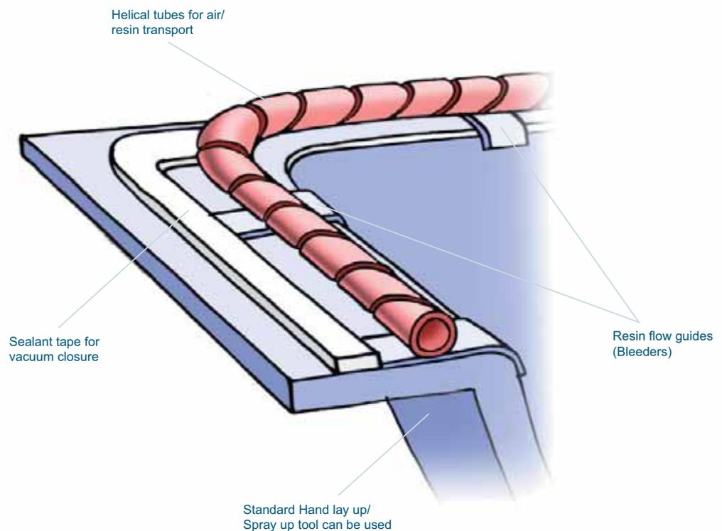
As with all composite mould designs sharp angles and corners should be avoided. De-moulding will be easier if certain draft angles and radius rules are applied at the part design stage. In infusion this is even more important as compacted reinforcement materials over sharp tooling edges can lead to resin flow problems and air entrapment. Aim for minimum 30° draft angles for parts less than 80 mm deep and 50° for deeper parts.
