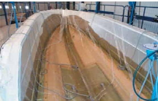
The plastic foil is kept in place and drawn down by vacuum. When the 'mould system' has been checked for possible leakages, the transfer of the resin can begin. The vacuum port and resin feed lines are connected to the system. As the required vacuum is reached, the resin reservoir is opened, and the resin flow starts.
