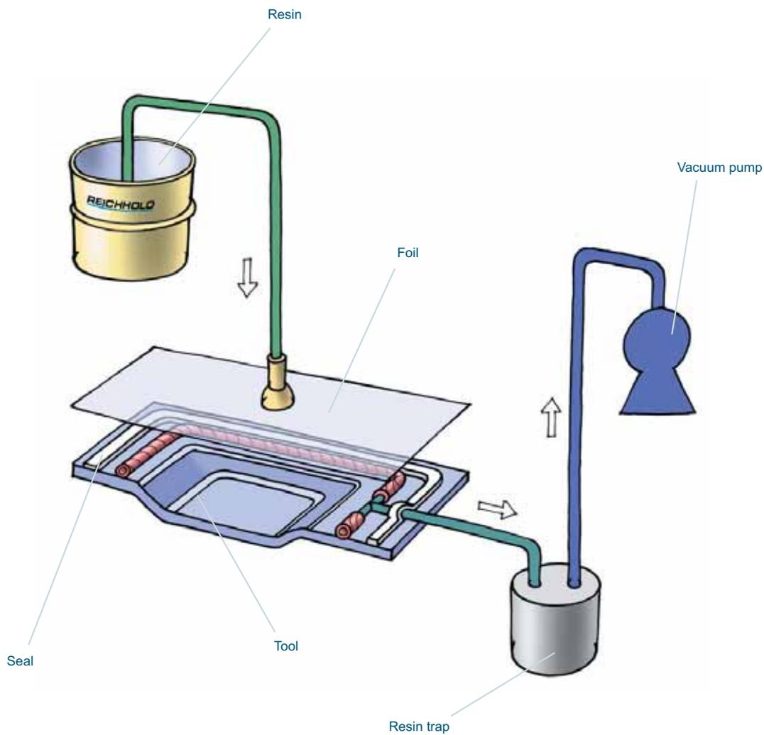
This guide will help to better understand the benefits and limitations of the Vacuum Foil Infusion processes and allow easier decision making on process parameters and key raw materials.
