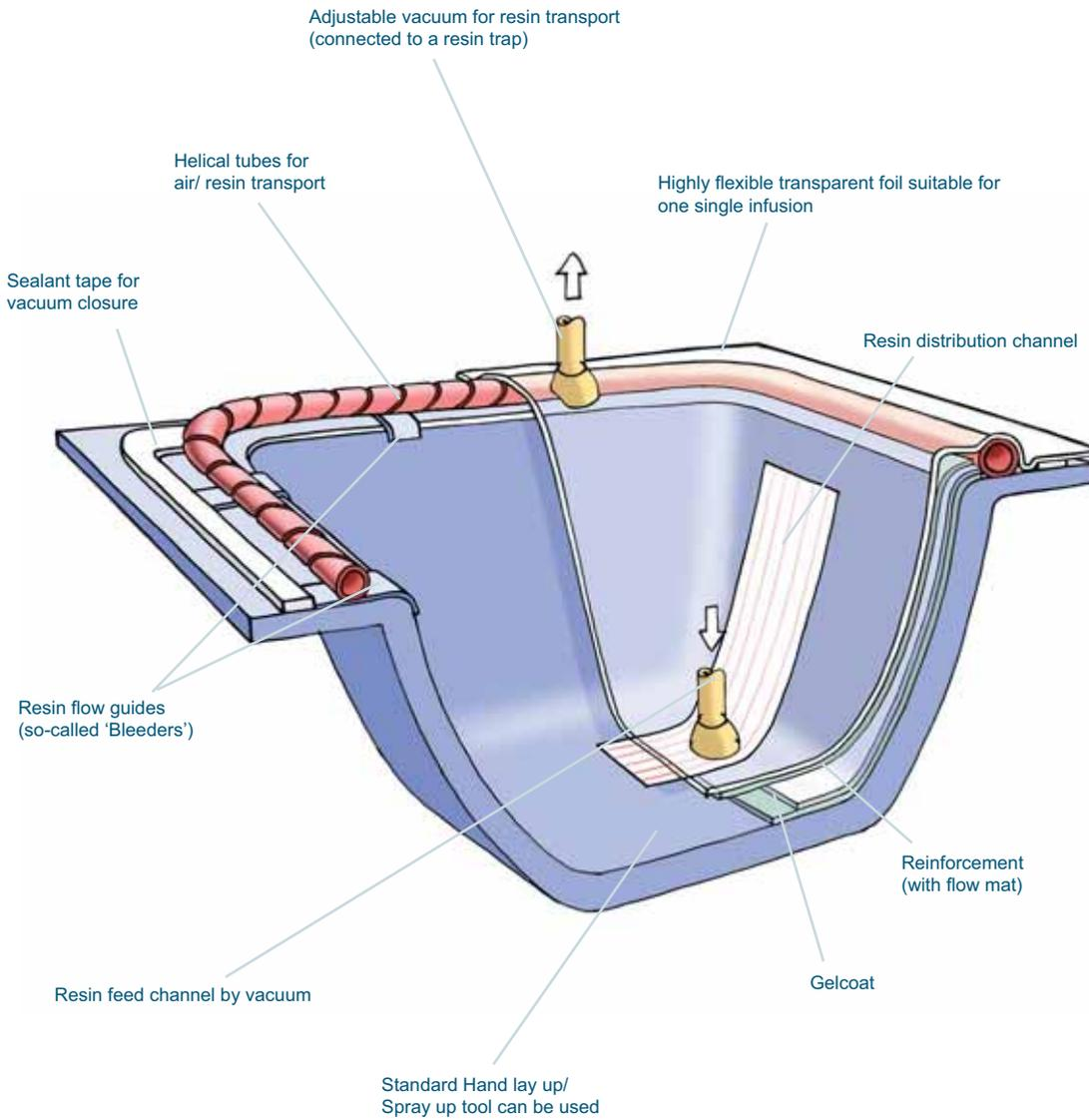
The Vacuum Foil Infusion method is typically considered cost effective for production of 50 - 1000 parts per tool per year.
