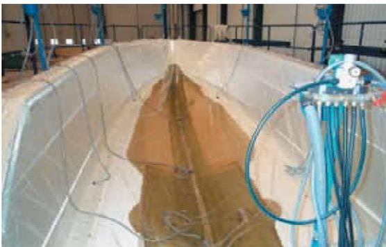
After the preparation of the mould (with mould release, gelcoat, barrier coat and/ or skin laminate), install the vacuum pump and resin trap; after placing the reinforcements and foil, the infusion process can start.
