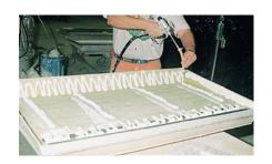
For surface treatment of GRP laminates, such as leveling uneven surfaces, the Norpol surface filler recommended is one that builds well, is easy to apply, offers quick curing and is easy to abrade.
