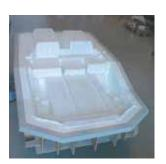
RTM Light is suitable for small production series of composites components of miscellaneous shapes and sizes with low investment outlay.
