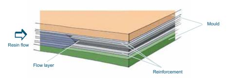
Different reinforcements can have different flow properties. In general there is an inversely proportional relationship between the flow properties and the mechanical properties. Finding the right balance between the two is often the best solution. For example one or more layers of a mat with good flow properties are placed in the core of the reinforcement package acting as a flow layer, whilst the rest of the reinforcements (e.g. chopped strand mat) will provide mechanical strength.
