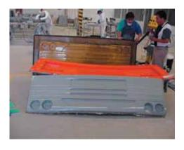
When the reinforcement package is fully impregnated with resin, the resin feed is cut off. Still under vacuum, the laminate is left to cure.
