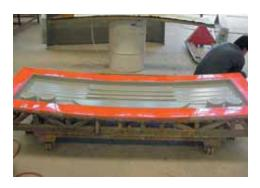
The process requires a rigid female mould and a semi-rigid male top mould. The mould closure occurs by applying vacuum aided by simple clamping mechanisms.
