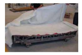
The resin is usually injected at low pressure (max. 1 bar) into a peripheral channel surrounding the part, and vacuum is applied to an exit port near the centre of the part.
