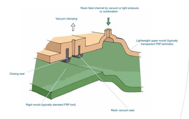
Two parallel rubber/ silicon seals are fixed in/ on the flange of the mould to enclose an area used for vacuum closure and the flange is equipped with vacuum connections to pull the closing vacuum between these seals.
