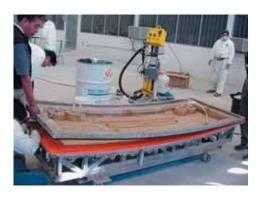
The low net closing pressure and low internal mechanical forces enable use of lightweight tools. For that reason it is possible to use tools similar (or adapted from) open moulding tools without significant extra investment.
